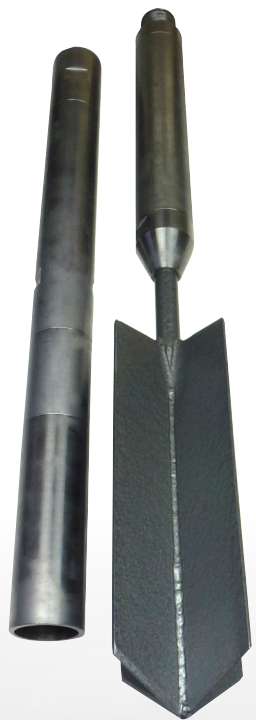
The new Envi Vane Shear Test System.
