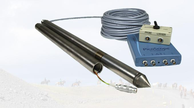
With the Seismic module you can perform insitu shear wave velocity measurement while you perform a Cone Penetration Test, thus in a cost effective manner.
