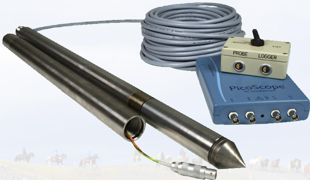
With the Seismic module you can perform insitu shear wave velocity measurement while you perform a Cone Penetration Test, thus in a cost effective manner.
