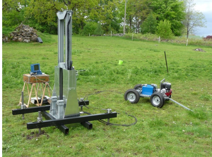
The Envi pusher. Can be transported on a pickup and manually moved when on site using the combined transport- and power pack trolley
