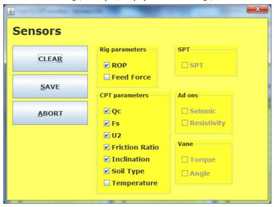
In order to start a sounding you first position the Memocone for start and then press START. You will then have a pop-up (see below) where you can set start depth for the sounding by scrolling value up and down with scroll wheels or enter an integer depth value in mm in the Depth text area. You save the start depth by pressing SAVE (keyboard command ALT+S). If you press ABORT no sounding will be started and you will return to the main window in the state you left it.
