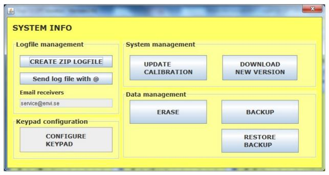
You create logfiles by pressing button CREATE ZIP LOGFILE. If the PC is connected to the logger system both calibration-/System data and logfiles will be zipped into the zip logfile that the system creates. If you are not connected to the logger system only the logfiles will be included in the zip logfile. You can choose where to save the zip logfile when the file dialog appears.
