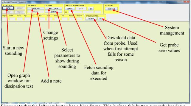
Please note that the leftmost button has a blue frame. This is since this button currently has focus and will be pushed if you have a keyboard and press Return or Space depending on your computer setup. To change button focus you use the TAB key (see below).
