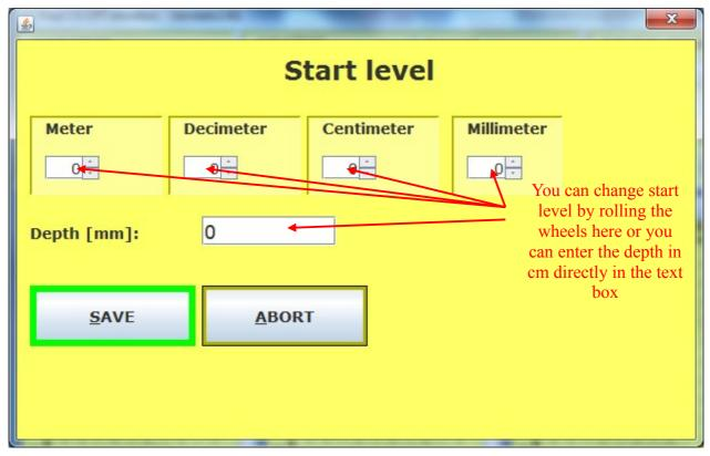
The system now starts to read and store sensor data. As soon as you have a change in depth graphs will start to be plotted. Measure values can also be seen in the different squares above and in graph window headers.
